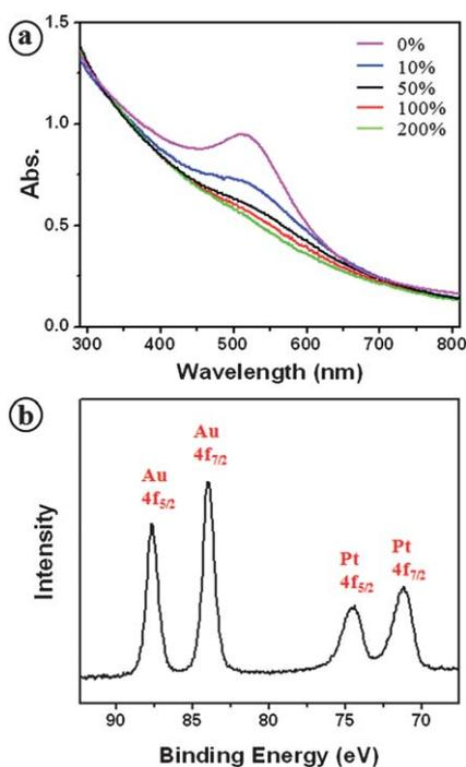
**Fig. 5** Characterization of shell-crosslinked Au-Pt nanoparticles. (a) UV-VIS spectra of Au nanoparticles hydroxylated with various mol % of Pt catalyst relative to the vinyl groups on the nanoparticle. (b)  $4f_{5/2}$  and  $4f_{7/2}$  XPS spectra of Au and Pt obtained from shell-crosslinked Au-Pt nanoparticles.
