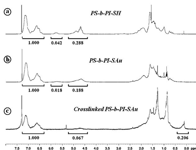
**Fig. 1** <sup>1</sup>H-NMR spectra of (a) PS<sub>29</sub>-*b*-I<sub>21</sub>SH, (b) gold nanoparticles coated by PS<sub>29</sub>-*b*-I<sub>21</sub>SH, (c) gold nanoparticles after crosslinking reaction of ligand.
