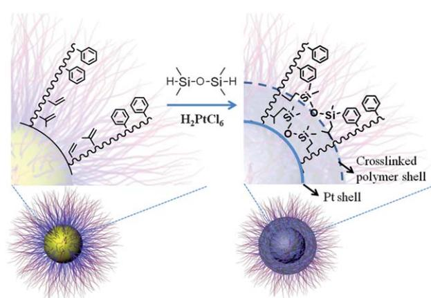
**Scheme 1** Schematic illustration of diblock copolymer ligands tethered to the surface of a gold nanoparticle and subsequent crosslinking of the vinyl-rich inner block *via* hydrosilylation with 1,1,3,3-tetramethyldisiloxane in the presence of platinum catalyst. The catalyst undergoes reduction on the gold surface during the reaction and forms a Pt shell.
