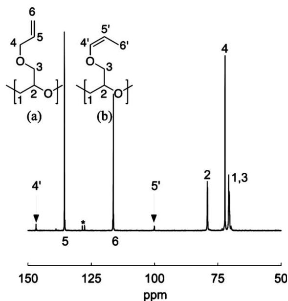
**FIGURE 4**  $^{13}\text{C}$  NMR spectrum of PAGE polymerized neat at  $120\text{ }^\circ\text{C}$  (see Table 2). Repeat unit isomers are shown with assignments in (a) and (b). Resonances due to carbon atoms in the benzyl end group are indicated with an asterisk.
