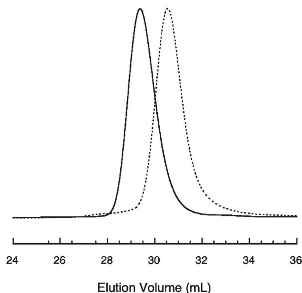
**FIGURE 2** Size-exclusion chromatograms of polymers 2 (dashed line,  $M_n = 11.8$  kg/mol, PDI = 1.08) and 6 (solid line,  $M_n = 27.5$  kg/mol, PDI = 1.07) as detailed in Table 1.
