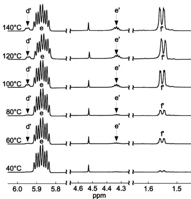
**FIGURE 5** <sup>1</sup>H NMR spectra resulting from polymerizations carried out at various temperatures (40–140 °C). All spectra are normalized to the intensity of the benzyl resonance near 4.5 ppm (2H), and peak-assignments are shown in Figure 3. The mole percent incorporation of *cis*-prop-1-enyl isomers increases with polymerization temperature for polymerizations of equivalent duration as evidenced by the increase in intensity of the peaks due to the d' (1H), e' (1H), and f' (3H) protons.
