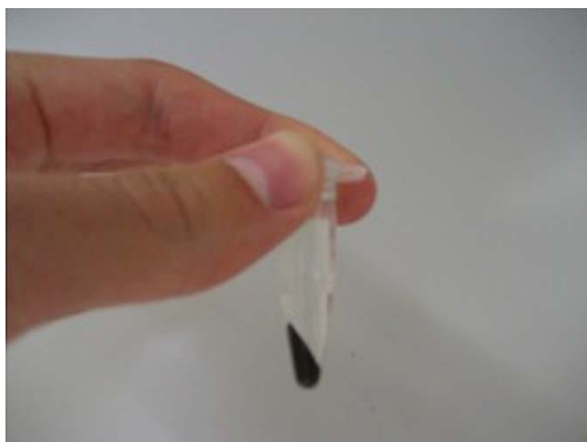
FIGURE 2 Representative image showing separation of CuNPs by centrifugation.
