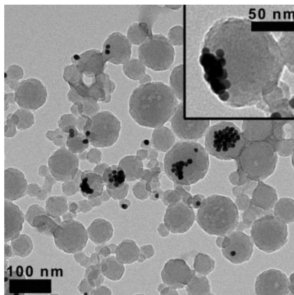
**FIGURE 2** Representative transmission electron micrograph from synthesis of composite polymer–gold nanoparticles using oleylamine-stabilized gold nanoparticles. Inset at top right shows both gold nanoparticle aggregation and incomplete encapsulation by polymer.
