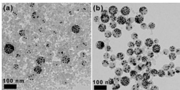
**FIGURE 9** Transmission electron micrographs illustrating the effect on composite nanoparticle formation of increasing the CTAB surfactant concentration to 17 mM, both before (a) and after (b) centrifugation to remove empty polymeric nanoparticles.
