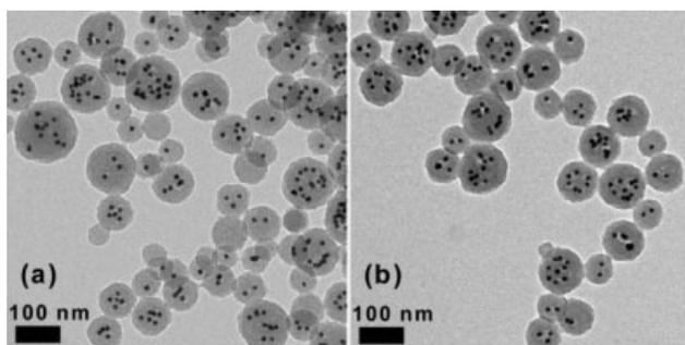
**FIGURE 11** Transmission electron micrographs of composite nanoparticles after redispersion in tetrahydrofuran (a), and after thiol-ene attachment of PEG and redispersion in chloroform (b).
