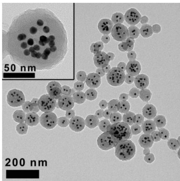
**FIGURE 3** Representative transmission electron micrograph of composite polymer–gold nanoparticles, showing 13 nm gold nanoparticles (black domains) encapsulated within larger, spherical poly(divinylbenzene) nanoparticles (gray domains). Inset at top left shows enlarged image of a single composite particle.
