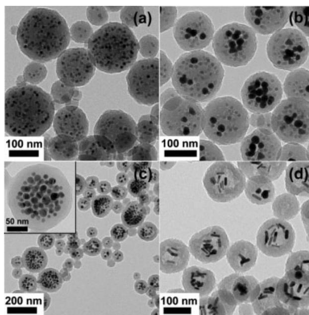
**FIGURE 12** Transmission electron micrograph of composite polymer- $\text{MnFe}_2\text{O}_4$  nanoparticles (a), hybrid polymer-gold- $\text{MnFe}_2\text{O}_4$  nanoparticles (b), composite polymer-silver nanoparticles (c), and composite polymer-gold nanorods (d).
