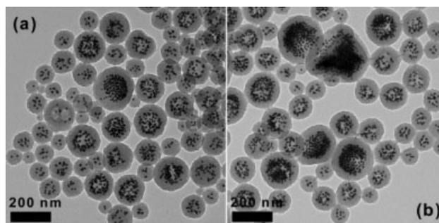
**FIGURE 7** Transmission electron micrographs of composite polymer-gold nanoparticles prepared with gold content of (a) 23 wt % and (b) 33 wt %.
