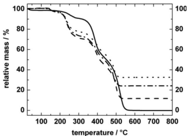
**FIGURE 6** Thermogravimetric analysis (TGA) of pure poly(divinylbenzene) particles (—), and composite poly(divinylbenzene)-gold nanoparticles with predicted gold loadings of ~12 wt % (---), 23 wt % (-·-·-), and 33 wt % (·····).
