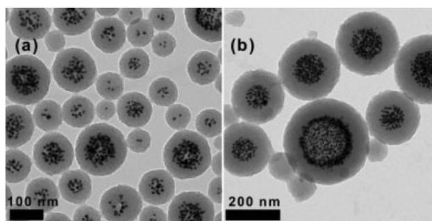
**FIGURE 8** Transmission electron micrographs illustrating the effect on composite nanoparticle formation of decreasing the CTAB surfactant concentration to (a) 0.57 mM, and (b) 0.17 mM.
