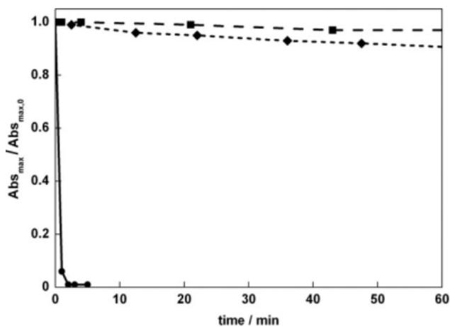
**FIGURE 5** Change in the relative UV-visible absorbance maximum after exposure to excess potassium cyanide for citrate-stabilized gold nanoparticles (—●—; 10 equiv of cyanide;  $\lambda_{\text{max}} = 520$  nm) and composite polymer-gold nanoparticles (---■---; 100 equiv of cyanide;  $\lambda_{\text{max}} = 550$  nm) in water, and for composite nanoparticles in 50/50 THF/water (---◆---; 100 equiv. of cyanide;  $\lambda_{\text{max}} = 550$  nm)
