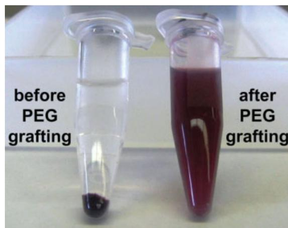
**FIGURE 10** Photographs of purified composite nanoparticles redispersed in THF and left to stand for 24 h (left), and following attachment of PEG surface groups by thiol-ene chemistry, redispersion in THF and left to stand for 24 h (right).
