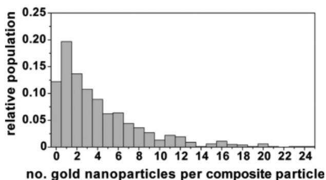
**FIGURE 4** Histogram showing the relative populations of composite nanoparticles containing different numbers of encapsulated 13-nm gold nanoparticles (compiled from TEM analysis of several hundred composite nanoparticles).
