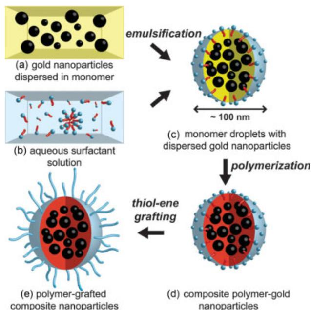
**FIGURE 1** Schematic description of composite nanoparticle synthesis: (a) polystyrene-grafted gold nanoparticles are dispersed in monomer (divinylbenzene) and emulsified with aqueous surfactant solution (b) to form small, uniform monomer droplets (c), which are then polymerized to yield composite polymer–gold nanoparticles (d); hydrophilic polymer chains (poly(ethylene glycol)) are grafted to the surface of composite nanoparticles by thiol-ene chemistry (e).
