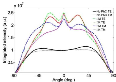
FIG. 4. (Color online) Comparison of the integrated intensity over wavelength for angular PL measurements in the  $\Gamma M$  and  $\Gamma K$  directions of PhC at TE and TM polarizations. All measurements were taken in the same conditions.
