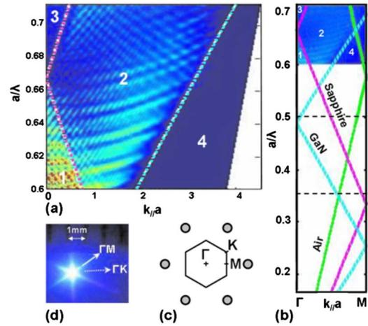
FIG. 2. (Color online) (a) Angular resolved PL measurements at 460 nm center wavelength in TE mode along the  $\Gamma M$  direction. (b) The same measurement on an expanded frequency scale. Green, magenta, and cyan lines correspond to light, sapphire, and GaN lines, respectively, in both figures. (c) First Brillouin zone of a hexagonal lattice. (d) A macroscopic picture of a PhC device excited by a UV laser.
