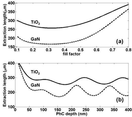
FIG. 3. PhC extraction length [ $L=1/2\text{Im}g(k||)$ ] obtained from numerical simulation comparing GaN and titania PhCs for the TE<sub>9</sub> mode in the  $\Gamma M$  direction as a function of (a) fill factor (defined as the ratio of the air hole volume over the PhC volume) and (b) the PhC depth.
