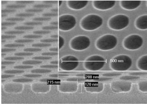
FIG. 1. PhC lattice of titania on a GaN LED substrate (inset: top view).
