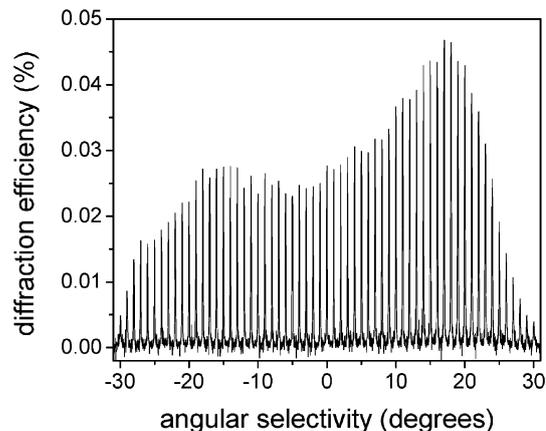
**Fig. 3** Angular selectivity curves of the 60 holograms recorded in 0.5 mm thick holographic disc containing second generation based monomer **3**.
