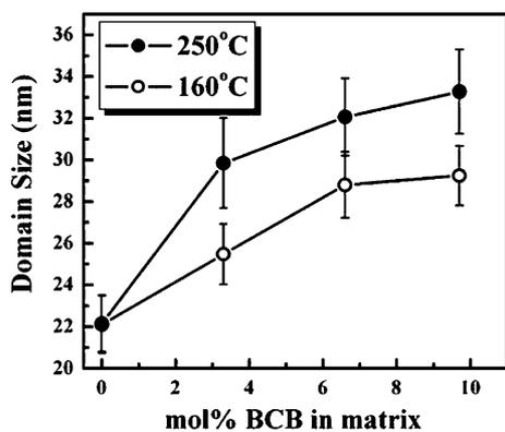
**Fig. 2** Domains size of PS-*b*-PMMA thin films with varying BCB amounts (0, 3.3, 6.6 and 9.7 mol%), annealed at 160 °C for one day and then further cross-linked at 250 °C for 15 min to prepare the entirely cross-linked thin films.
