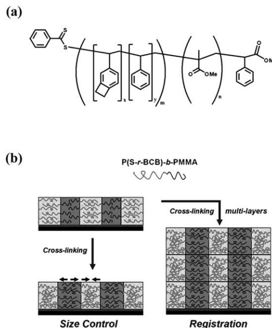
**Scheme 1** (a) Molecular structure of (PS-*r*-BCB)-*b*-PMMA copolymers and (b) schematic for the cross-linking process and multi-layer registration of the BCP thin films. The benzocyclobutene (BCB) functionality is randomly incorporated into the PS block with the different BCB amounts (3.3, 6.6 and 9.7 mol%).
