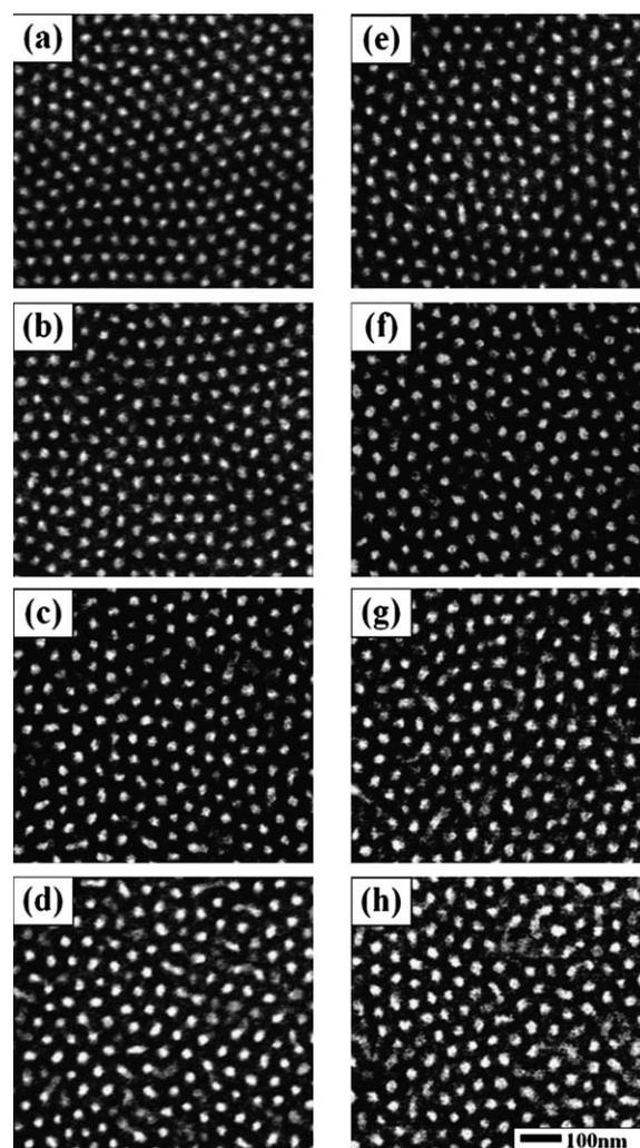
**Fig. 1** TEM images of PS-*b*-PMMA thin films with varying BCB amounts (0, 3.3, 6.6 and 9.7 mol%). The left and right images were taken from thin films annealed at  $160^\circ\text{C}$  for one day and subsequently cross-linked at  $250^\circ\text{C}$  for 15 min. The microdomains of the PS-*b*-PMMA were oriented normal to the surface due to the balanced interfacial interaction on the surface by the random copolymer brush.
