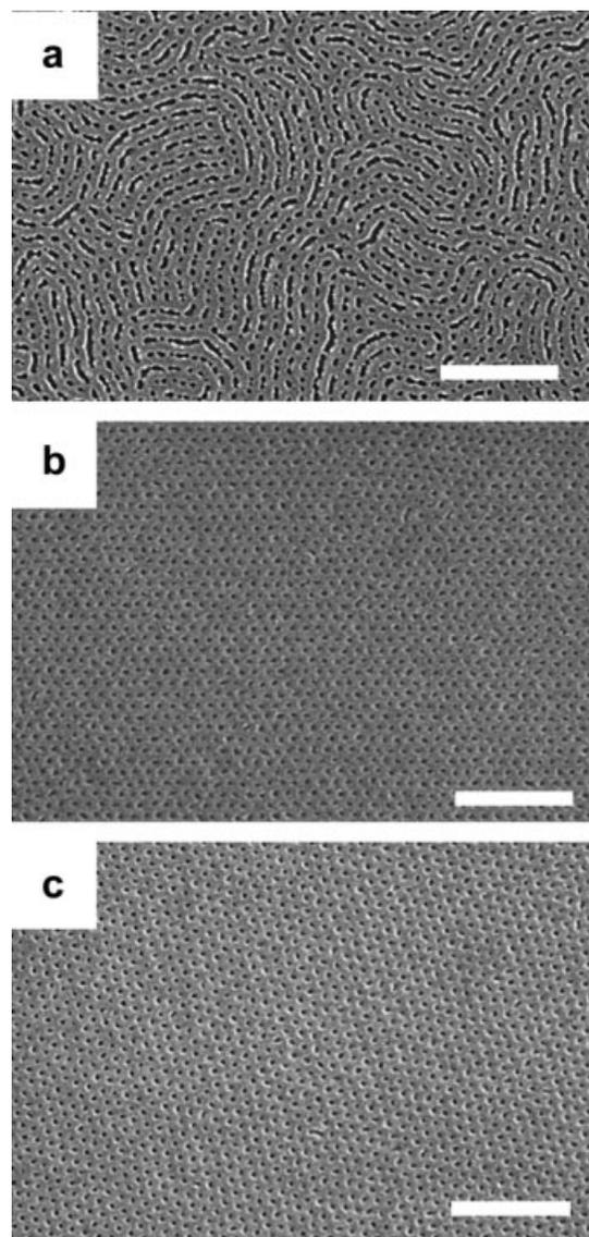
**Figure 2.** SEM images for PSt-*b*-PMMA thin films containing 5.0 wt % of PEO star polymers, (a) EO-S2(4), (b) EO-S7(8), and (c) EO-S16(8). All experimental conditions are same as Figure 1. Scale bars are 500 nm.
