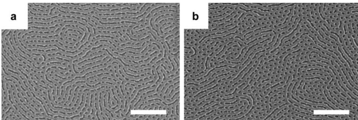
**Figure 3.** SEM images for PST-*b*-PMMA thin films containing 5.0 wt % of linear PEO homopolymers, (a) EO-H4 and (b) EO-H10. All experimental conditions are same as Figure 1. Scale bars are 500 nm.
