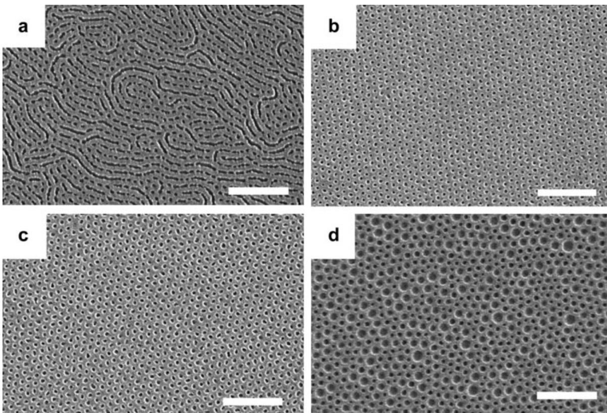
**Figure 1.** SEM images for PSt-*b*-PMMA thin films containing (a) 1.0 wt %, (b) 3.0 wt %, (c) 5.0 wt %, and (d) 10.0 wt % of EO-S100(20) after solvent annealing under high humidity conditions ( $\sim 90\%$ ), followed by UV treatment and rinsing with acetic acid to remove PMMA microdomains. Scale bars are 500 nm.
