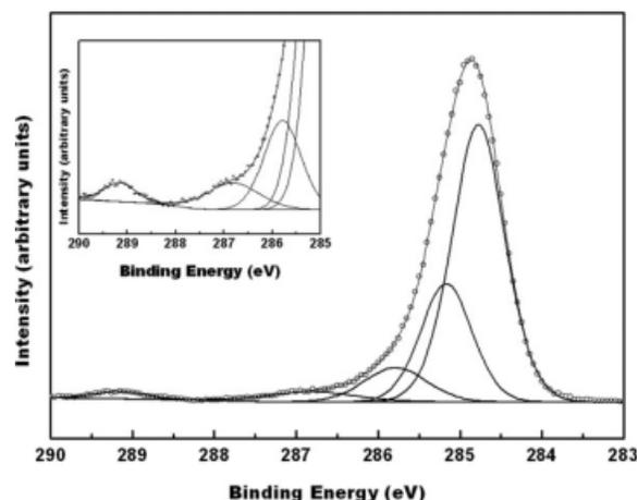
**Figure 4.** High resolution XPS spectra for PST-*b*-PMMA thin films containing 5.0 wt % of EO-S16(8) after solvent annealing under high humidity conditions (~90%).
