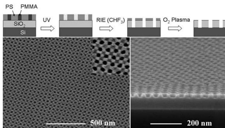
**Fig. 5.** (Top) Schematic representation of pattern transfer from supramolecular block copolymer thin films; PEO domains are omitted for clarity. (Bottom) SEM top view and  $75^\circ$  cross-section images of square arrays of cylindrical pores in silicon oxide after RIE and  $\text{O}_2$  plasma treatment of a UV-degraded thin-film blend of supramolecular block copolymers **1** and **2a**. (Inset) Magnified SEM top view.
