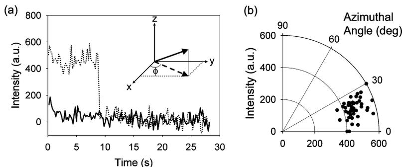
**Figure 2.** A molecule whose orientation is essentially fixed. (a)  $I_x$  (···) and  $I_y$  (—) as functions of time. (b) Corresponding in-plane orientation angle,  $\phi$ , of this molecule during the time it is emitting light. These figures are for a center-labeled PB chain in PB. Inset: experimental reference frame showing  $\phi$  relative to the two polarization axes,  $x$  and  $y$ , and the laser propagation axis,  $z$ .
