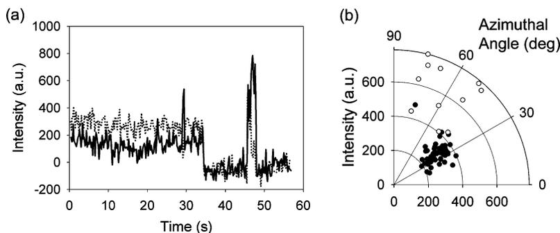
**Figure 3.** A molecule that blinks and changes orientation. (a)  $I_x$  (···) and  $I_y$  (—) as functions of time. (b) Corresponding in-plane orientation angle,  $\phi$ , of this molecule during the first (●) and second (○) on-times. These figures are for a center-labeled PB chain in PB.
