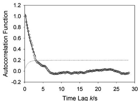
**Figure 4.** A sample plot of an autocorrelation function as a function of lag time. The confidence limit, defined by the standard error, is also included (···). A single-exponential fit is shown for the statistically significant points (—). This figure presents the ACF of the total emitted intensity for a center-labeled PI chain in PI, and the exponential decay fit has a decay time of  $1.9 \pm 0.05$  s.
