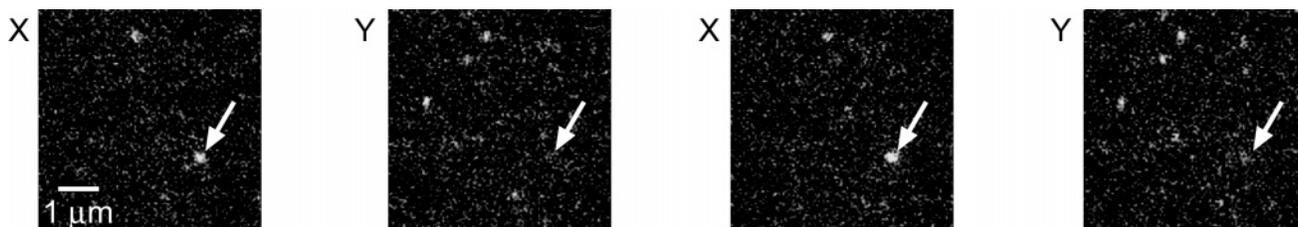
**Figure 1.** Sample images of polymer-tethered perylene molecules taken using the polarization-modulated epifluorescence configuration described in the text. These are consecutive images, separated by 100 ms and illuminated with light of two orthogonal polarizations in the  $X$ - $Y$  plane. The arrow indicates a molecule that is excited by only one polarization due to its orientation.
