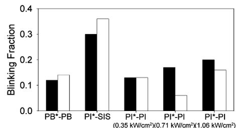
**Figure 6.** Bar graph comparing the fractions of molecules that blink during the course of observation for each experimental system. In general, there are no clear trends between center- (black) and end-labeled (white) chains or as a function of illumination intensity. However, a higher fraction of the dyes in the SIS host blink compared to any of the other systems.
