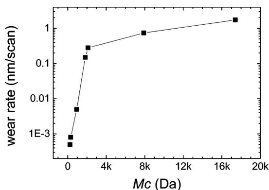
**Figure 4.** Impact of cross-link spacing on wear rate. Two wear regimes are separated by a critical molecular weight between cross-links,  $M_c$ . Below  $M_{c,crit} = 2150 \pm 150$  Da, wear is highly sensitive to the cross-link density, while above 2150 Da, there is little wear dependence on  $M_c$ . The uncertainty level represents the intersecting domain defined by the root mean square variance of regression fits above and below  $M_{c,crit}$ .
