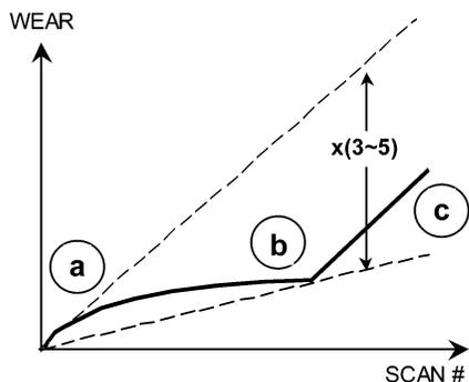
**Figure 3.** Schematic wear diagram: typical behavior represented by the solid line. The dominant wear mode changes during the course of the experiment, from (a) an initial rapid ripple formation to (b) an apparent static rippled state which ends abruptly with the onset of (c) rupture wear and abrasion. This evolution of wear modes leads to a long-term wear rate that is distributed between two extremes (given by the slopes of the dashed lines) separated by a factor of  $\sim 3\text{--}5$ .
