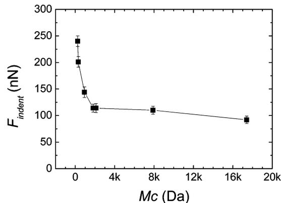
**Figure 5.** Impact of cross-link spacing on the hardness of the PS–BCB thin films: The minimum force needed to make a permanent 0.5 nm deep indentation,  $F_{indent}$ , is plotted versus the molecular weight between cross-links,  $M_c$ . (Note: for a given indentation geometry and penetration depth (i.e., equal contact area), the hardness is directly proportional to  $F_{indent}$ .)
