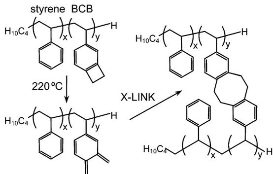
**Figure 1.** A cross-linking mechanism for random styrene–benzocyclobutene copolymers (PS–BCB), with a BCB content ( $y$ ) varying between 0 and 30%.
