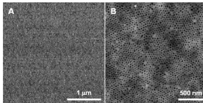
**Figure 2.** A) Phase contrast AFM image of the surface of PS-*b*-PMMA/PMMA film. The image shows an area of 3 μm × 3 μm. B) Height contrast AFM image of the surface of the identical film in (A) after PMMA microdomains were removed by UV exposure and acetic acid rinsing. The image shows a 2 μm × 2 μm area on the surface.
