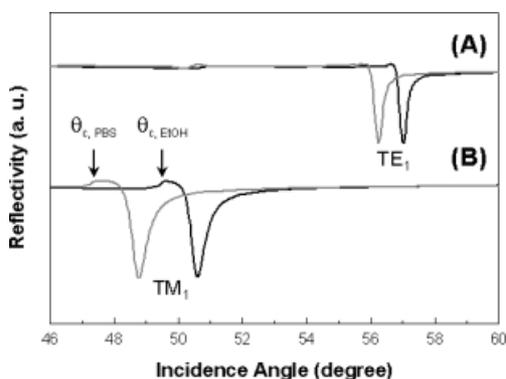
**Figure 4.** Waveguide mode patterns of the porous PS template filled with a pH 7.4 PBS solution (gray lines) and in ethanol (black lines) under s-polarization (A) and p-polarization (B), respectively. The critical angles under PBS and ethanol environments are marked by arrows.
